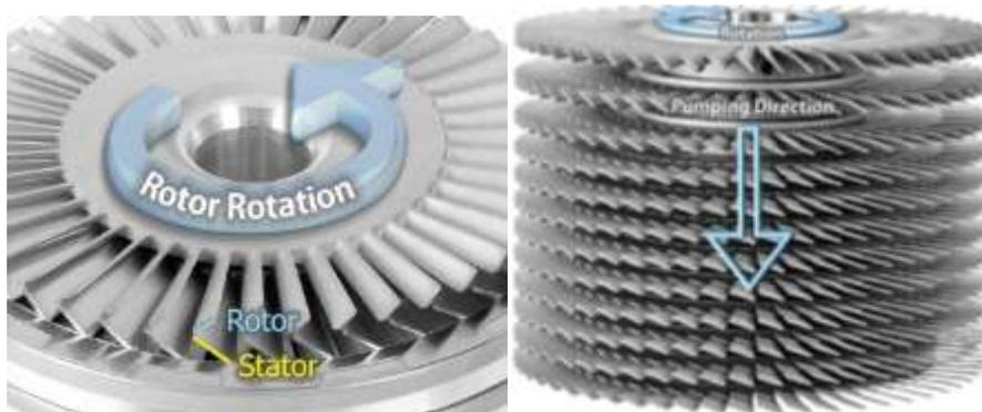
Fig. 2.19: A) Diagram showing the arrangement of the rotor and stator blades. B) The rotor blades of the turbo pumps down gas molecules out of the chamber<sup>33</sup>.
