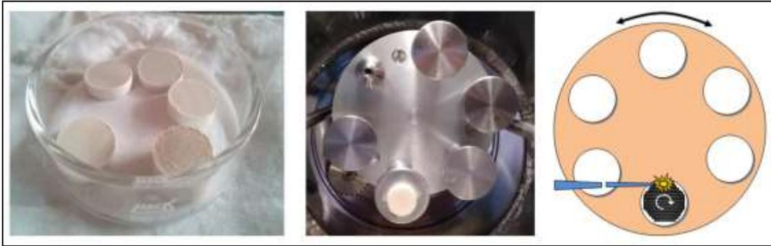
Fig. 2.3: A)  $\text{TiO}_2$  pellets. B) The pellet is mounted on the stub which is attached to carousel disc. C) Schematic diagram of the target carousel showing the motion of both target and the disc which is holding the target.
