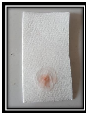
Fig:24(b) Indicator strip used to detect presence of iron in water collected from well near field
