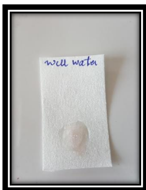
Fig:24(c) Indicator strip used to detect presence of iron in water collected from well in the city.
