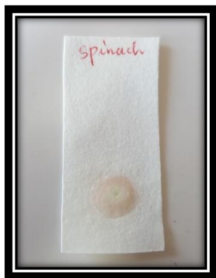
Fig:23 paper strip showing presence of iron in spinach
