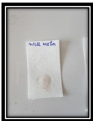
Fig:24(a) Indicator strip used to detect presence of iron in water collected from well near river.
