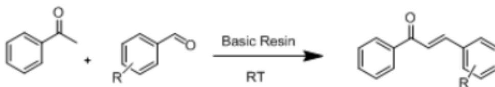
Equation 4 Synthesis of chalcones using ion exchange resin
